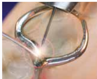
repair of broken clasp
