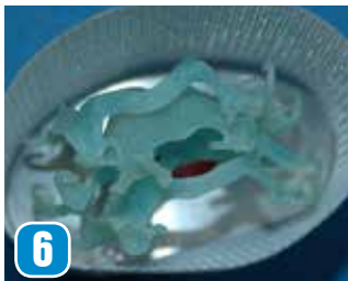
6 when using the Metaring investing system three partials can easily be cast in one ring
